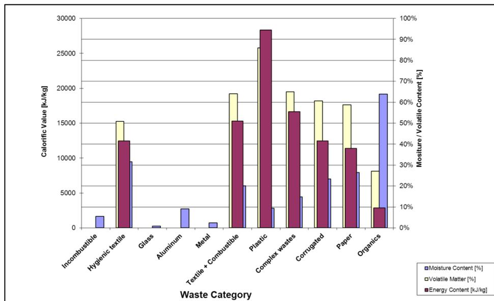
Figure 2: Mean moisture, volatile content and calorific value of each waste category of Amman City
